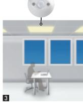
Presence detected, insufficient daylight, all lights on
