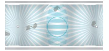
**PIR detection** should be given preference. It provides good detection performance for people moving around, with a long detection range.
