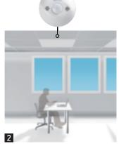
Presence detected, sufficient daylight, lights off
