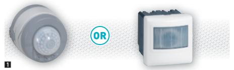
**Cat.No 0 697 40** Adjustable PIR motion sensor Directional head to detect people mounting stairs 360° Range Ø 8 m IP 55 Surface-mounting on wall or ceiling (one sensor per floor).
